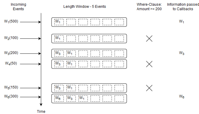
Figure 2.9. EPL Basic Where-Clause Example Input and Output Flow
